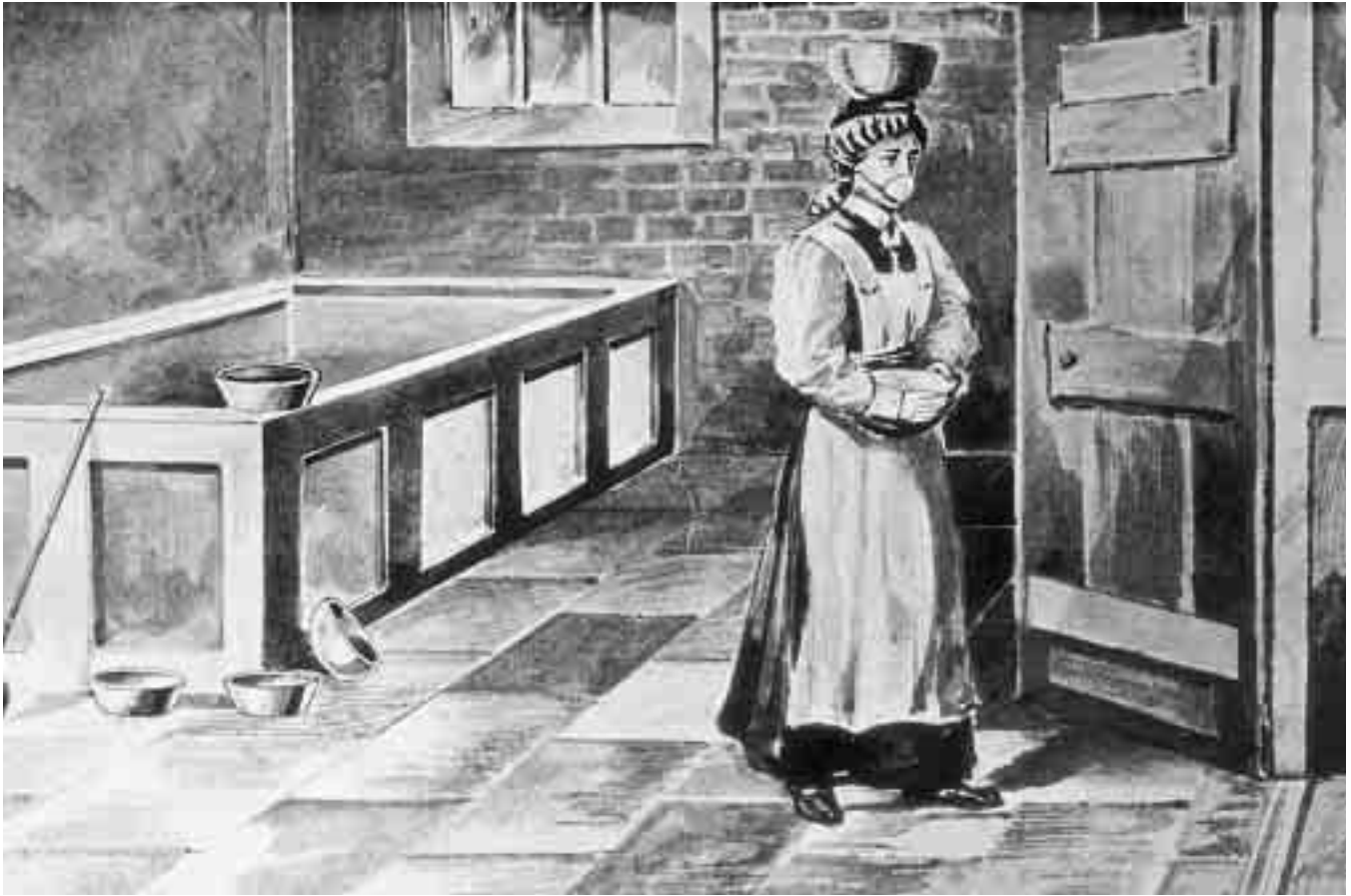
Lead poisoning: female carrying basins filled with washed white lead from vats to stoves, 1902
